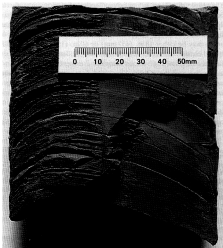
Fig. 7.4 Heavy shear distortion in a clay sample taken using a driven BS U100 sampler with a plastic liner (courtesy Surrey Geotechnical Consultants Ltd).
